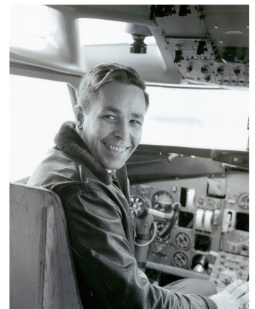
Lew Wallick in original 727 cockpit days before 1 st flight (note temporary plywood seat back and missing instrumentation)
